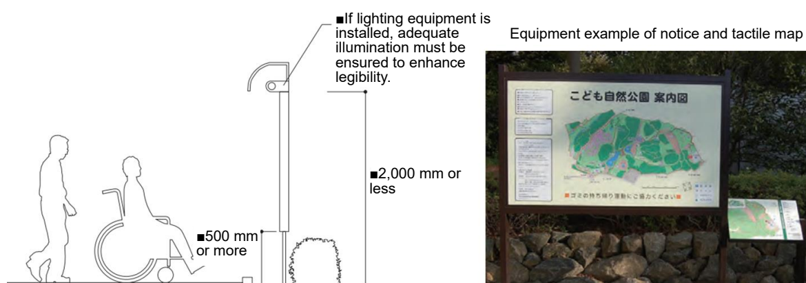
Figure: Example of notice installation (indoor)
